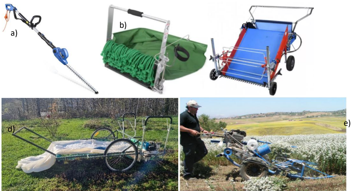
Figure 20: a) long-reach edge trimmer (HYINDAI Power products, n.d.), b) handheld tool with macrame braided string pick-up reel (Terrateck, n.d.-c), c) hand pushed, powered harvesting method with conveyor belt transport mechanism (Terrateck, n.d.-b), d) Japanese tea harvesting machine with airflow transport mechanism, adapted with construction and tires to be used by one person (Zermanek Biohof), e) Reaper-binder (Comparetti et al., 2022)
