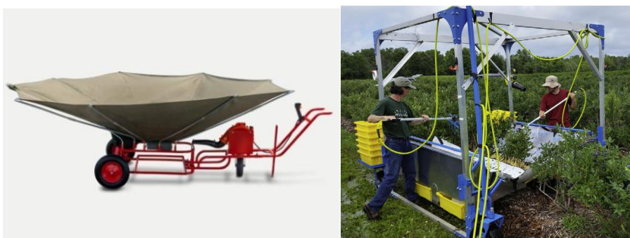
Figure 18: Upside down umbrella catching mechanism (left, (HARVEST, n.d.)), Semimechanical harvester for blueberry (right, (Zhou et al., 2016))
