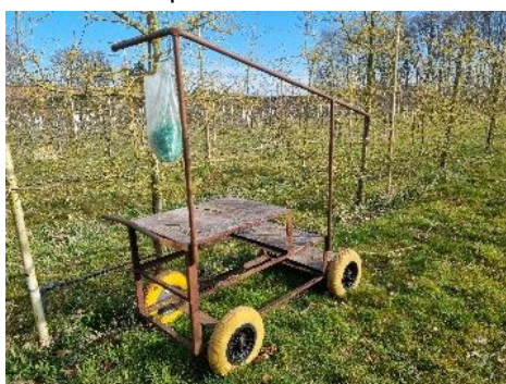
Figure 48: Self built step ladder with wheels for fruit harvest (De walnoothoeven)
